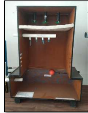
Induced draught cooling tower by SYME students- Sameer Mansuri, Omkar Singh, Ashmit Chhajalana & Vishal Vishwakarma
