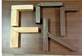
Bend Square Pipe at Right Angle without Removing Material
